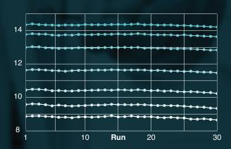
The retention times of the 7 peptides analysed in the adjacent figure were plotted across 30 runs to demonstrate retention time stability for the Aurora Rapid75<sup>TM</sup> column.
