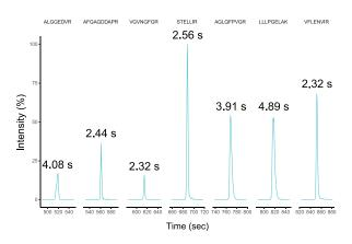
A HeLa tryptic digest (1 ng) was separated on an Aurora Rapid75™ column using a Thermo Scientific Vanquish Neo UHPLC and TSQ Quantis across a 15 min sample gradient at 100 nL/min. The extracted ion chromatograms for 7 selected peptides from the analysis are shown. The average Full Width at Half Maximum (FWHM, seconds) for each peptide across 30 runs is shown above each peak.
