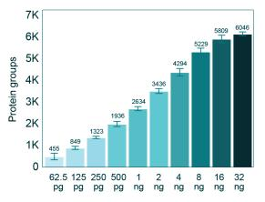
A dilution series of a HeLa tryptic digest was separated on an Aurora Rapid75™ column using an Evosep One and Bruker timsTOF SCP (dia-PASEF) using an 80 samples per day method (currently under development), n = 6. Data courtesy of Dr Christoph Krisp (Bruker), Dorte Bekker-Jensen and Dr Nicolai Bache (Evosep).
