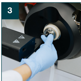
3 Unscrew the emitter lock anti-clockwise.
