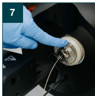
7 Using a gloved finger, block the air inlet and monitor the fore pressure. The fore vacuum needs to drop to below 3e-01 mbar within 10 seconds to be considered usable.
