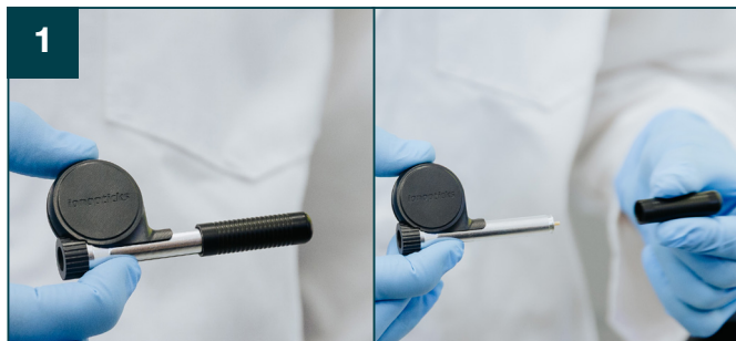
1 Remove cap from the HeatSync ™ Rapid 5 cm Column Housing.
