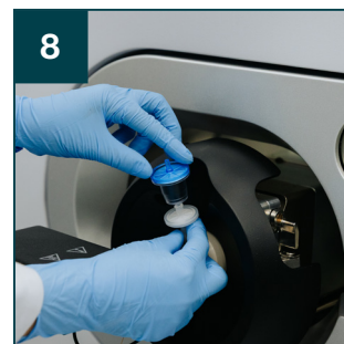
8 Install filter into the CaptiveSpray source air inlet.
