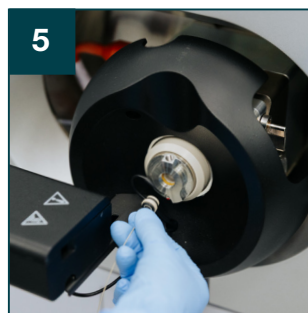
5 Carefully insert the CSI fitting into the CaptiveSpray source in a single motion (do not twist)
