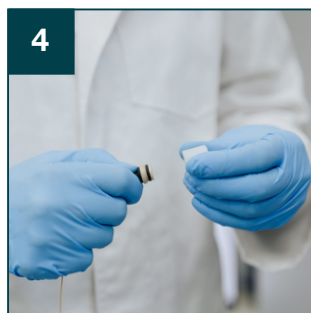
4 Carefully remove the CSI Protective cap.
