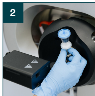
2 Remove the filter from the CaptiveSpray source air inlet.
