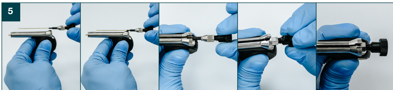
5 Slowly lower the column through the opening and slot. Once the column is in the slot and the end of the protective sleeve is aligned with the small hole at the end of the slot, push it forward. Ensure the NanoZero is positioned correctly — the horizontal edge should be centered within the opening, as shown in the image.
