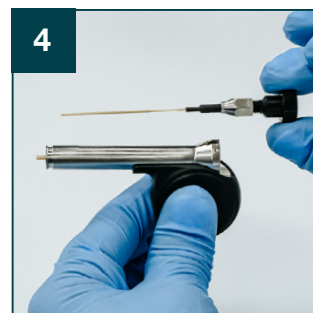
4 Hold the column with the shipping plug attached, as shown in the image.
