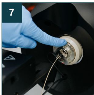
Using a gloved finger, block the air inlet and monitor the fore pressure. The fore vacuum needs to drop to below 3e-01 mbar within 10 seconds to be considered usable.
