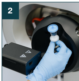
Remove the filter from the CaptiveSpray source air inlet.
