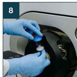
Install filter into the CaptiveSpray source air inlet.
