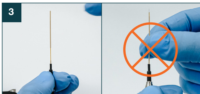
3 Take the Aurora 5 cm Rapid column and ensure that the beige protective sleeve is protecting the emitter.
