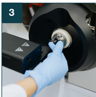
Unscrew the emitter lock anti-clockwise.
