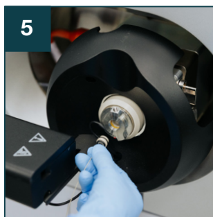
Carefully insert the CSI fitting into the CaptiveSpray source in a single motion (do not twist)
